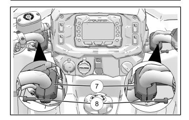
4. Install the windshield assembly onto the mounting clamps and take time to position the mounting clamps and adjust the windshield to the headlight pod. Tighten both windshield mount adjuster screws and torque the mounting arm fasteners (6) and mounting clamp fasteners (8) to specification once the windshield is in place.
