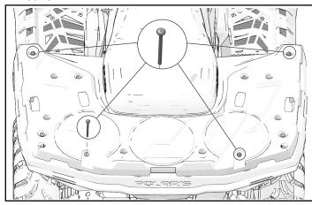
2. If equipped with dual tail lamps, unscrew the tail light shield on the right side and move shield aside.
