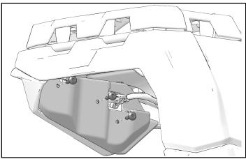
3. Align rear rack extender on rear box cover.
