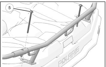
6. Install nut 6 onto screw 5. Repeat other side. Torque screws to specification.
