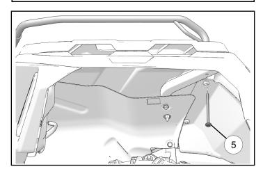
5. Install two screws (5) through the rear rack extender down through the box cover.
