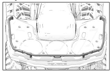
4. Install screw ⑤ from the underside of box cover up into rear rack extender. Repeat other side. Torque screws to specification.
