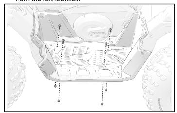
3. Install the left-hand bracket mount (1) onto the left footwell. Loosely install the two front footwell screws (3) and nuts (9) to hold the assembly into place.
