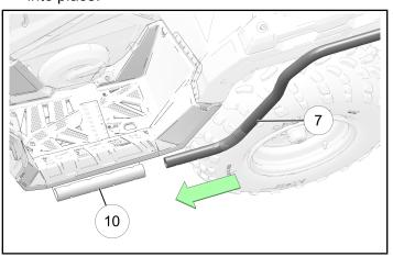
5. Align the bracket on the rear left-hand side guard weld ① with the rear rack tube support. Loosely install the nut that was previously removed in step 1 to hold the bracket and the rear rack tube support into place.
