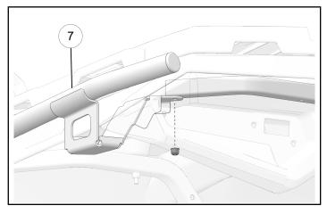
6. Loosely install the two rear footwell tube screws ④ and nuts ⑫ to hold the assembly into place.
