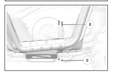
8. Slide the front left-hand side guard weld ① into the left-hand bracket mount ⑩ and lift the assembly into place.
