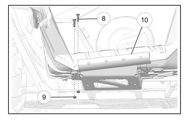
4. Slide the rear left-hand side guard weld ① into the left-hand bracket mount ⑩ and lift the assembly into place.
