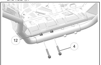
10. Align the front left-hand side guard weld ① with the front left side of the applicable front bumper kit. Install the bumper screw ② through the front bumper and into the front left-hand side guard weld ①.
