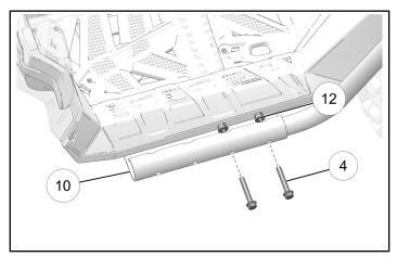
7. Loosely install the two rear footwell screws ® and nuts 9 to hold the assembly into place.
