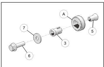
4. While ensuring slider is firmly seated against vehicle frame, and flats are properly aligned, tighten screws ⑥. Torque screws to specification.
