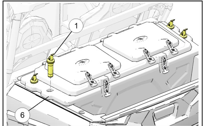
4. Depress expansion anchor ① cams to lock storage box ⑥ in bed as shown. If installation is loose, remove anchor from box, tighten nut at anchor base, and reinstall.
