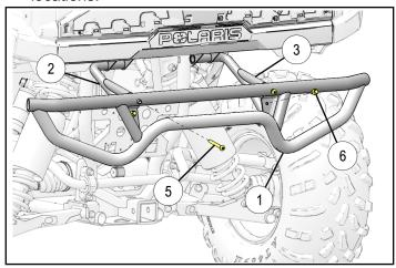
4. Lift bumper ① as high as possible, then torque all eight screws to specification.
