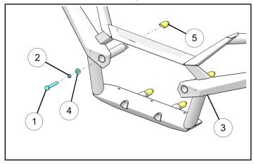
Install bumper assembly ③ onto front fascia (A) by inserting four wedge mounts into the holes in fascia. Push on bumper and tighten all four screws ①.
