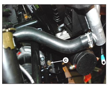
3. Check that contact or wires are clearing the fan shroud and any other frame members close by.
